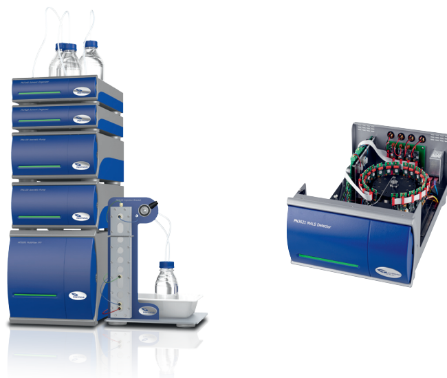
Figure 1: Experimental setup: Postnova AF2000 Asymmetrical Flow Field-Flow Fractionation system (left); Postnova MALS detector (right).
