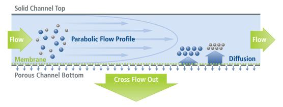
Figure 1: Schematic of AF4 principle.
