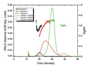
Figure 3. The ratio of  $R_a/R_b$  plotted across each peak in the fractogram.
