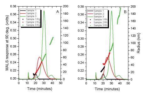
Figure 2. Fractograms with MALS response at 90°, with dots across each peak representing  $R_n$  (Figure 2A) and  $R_h$  (Figure 2B.)
