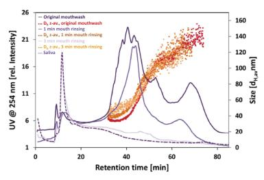
Figure 1: AF4-UV-DLS fractograms of the four samples showing UV signals (lefthand y-axis) vs. elution time, with overlaid sizes (Dh, z-average, right-hand y-axis).
