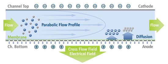
Figure 1: Schematic of EAF4 channel. In addition to hydrodynamic size separation via the flow field, an electric field allows for further separation by a molecule or particle's surface charge.
