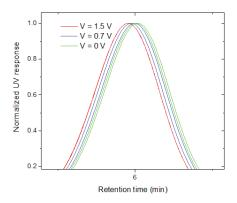
Figure 4: NIST mAb retention time shift with applied electric field.
