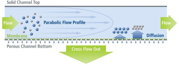
Figure 1: AF4 separation principle
