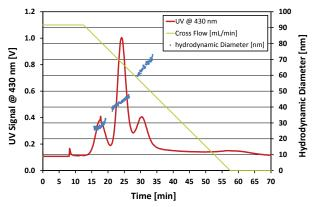
Figure 3: AF4-DLS fractogram of a 1:1:1 (w%) mixture of AgNP (20 nm, 40 nm, 60 nm)
