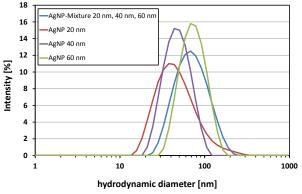
Figure 2: Comparison of intensity-based particle size distributions for single AgNP and AgNP in a 1:1:1 (w%) mixture obtained from DLS in batch mode.
