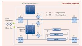
Fig. 4: Principle of Viscosity Detection.
