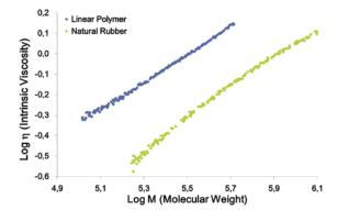
Fig. 6: Mark-Houwink-Plot of a linear polystyrene (blue line) and a slightly branched natural rubber sample (green line).
