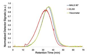
Fig. 5: TF3 Fractogram of a linear polystyrene sample with a broad distribution (blue: MALS, red: ELSD, green: Viscometer).
