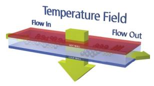
Fig. 1: Principle of Thermal Field-Flow Fractionation.
