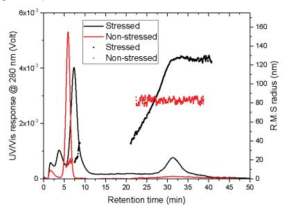
Figure 3: UV-based fractogram (black and red traces) overlaid with R<sub>a</sub> values (black and red dots) for two different AAV samples.
