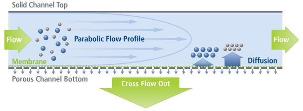
Figure 1: Principle of Asymmetrical Flow Field-Flow Fractionation.
